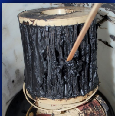
Filter clogged by Microbial / Fungal contamination aka 'Diesel Bug'
