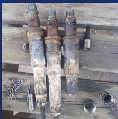
Seized Injectors after prolonged use with Fuel contaminated by Illuminated Paraffin.
