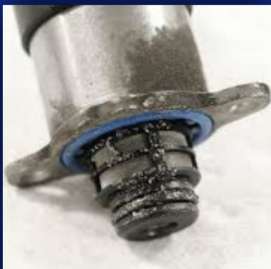
Abrasive metal particles found in Diesel fuel system, caused by Diesel with adulterated lubricity.
