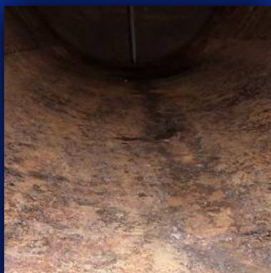
Corrosion inside underground fuel storage tank - caused by water attracted to hygroscopic Ethanol.
