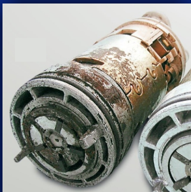
Fuel System damage caused by water contamination.
